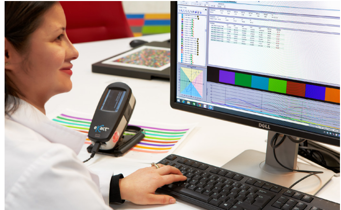
SunColorQC is a software platform hosted on the Sun Chemical network that uses software and a connected spectrophotometer to measure the quality of the output on press.
